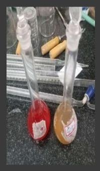
Take 20 ml of solution from the measuring flask into a titration flask add 20 ml of dil. H2SO4 to it.
