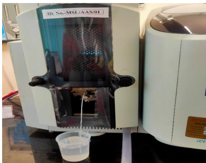
Burning of Nitric acid solution in AA Spectrometer
