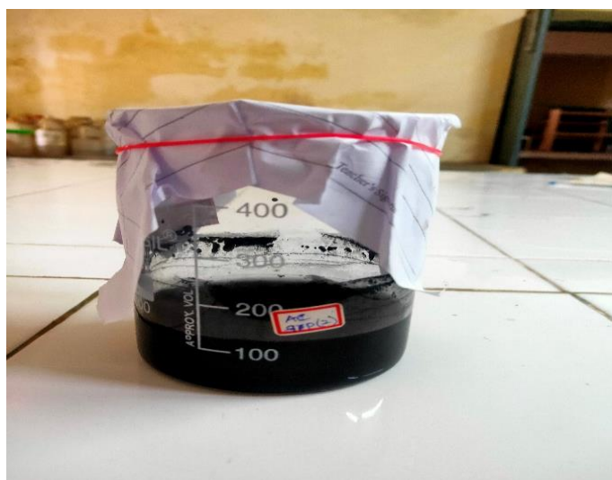
5gm of Activated charcoal in metal ligand solution
