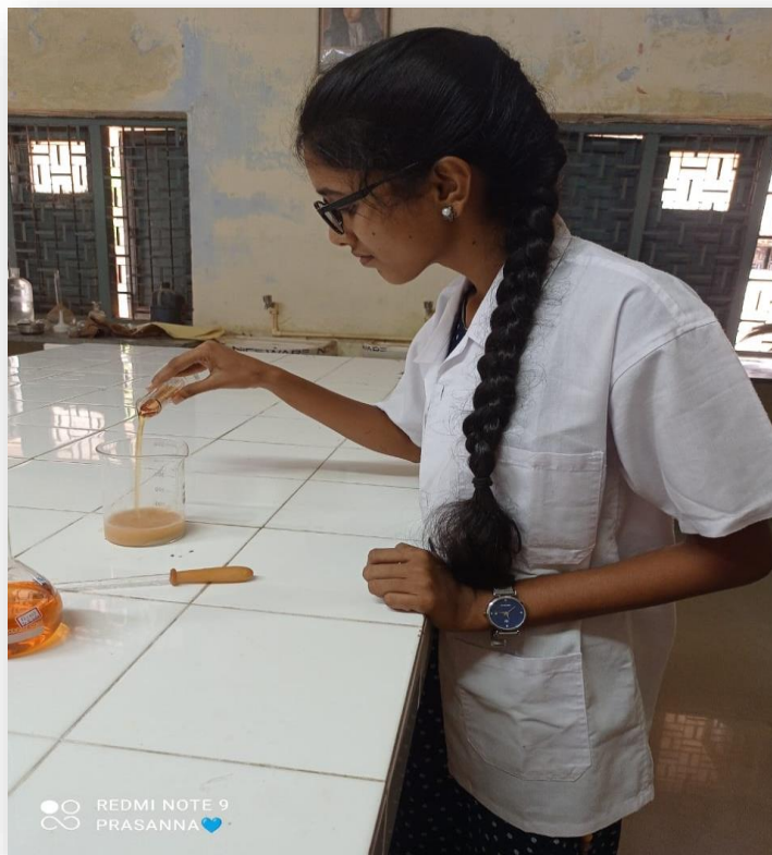
Addition of Celite to Metal-Ligand Solution
