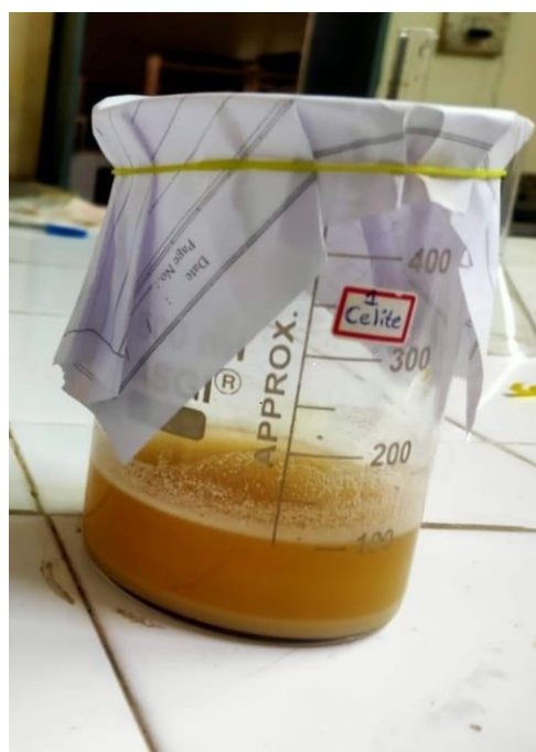
Cellulose added to Metal Ligand solution is prepared
