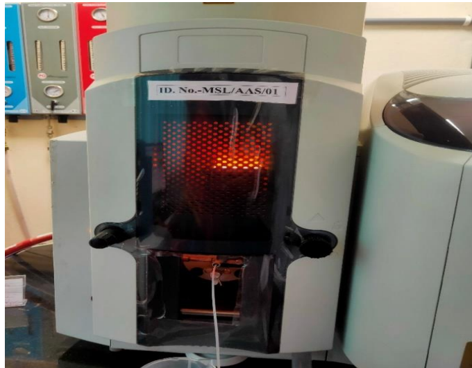
Burning of Test sample in AA Spectrometer
