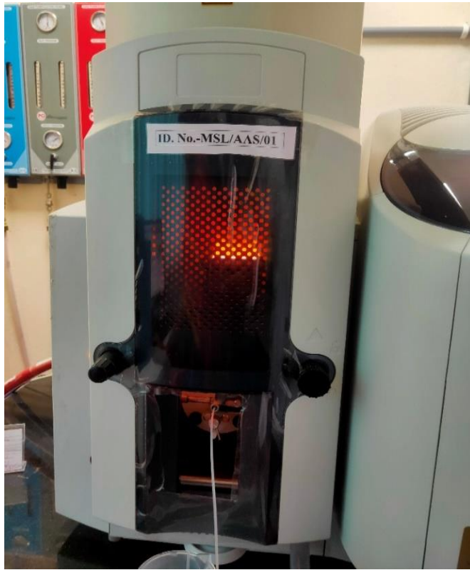
Burning of test sample in AASpectrometer
