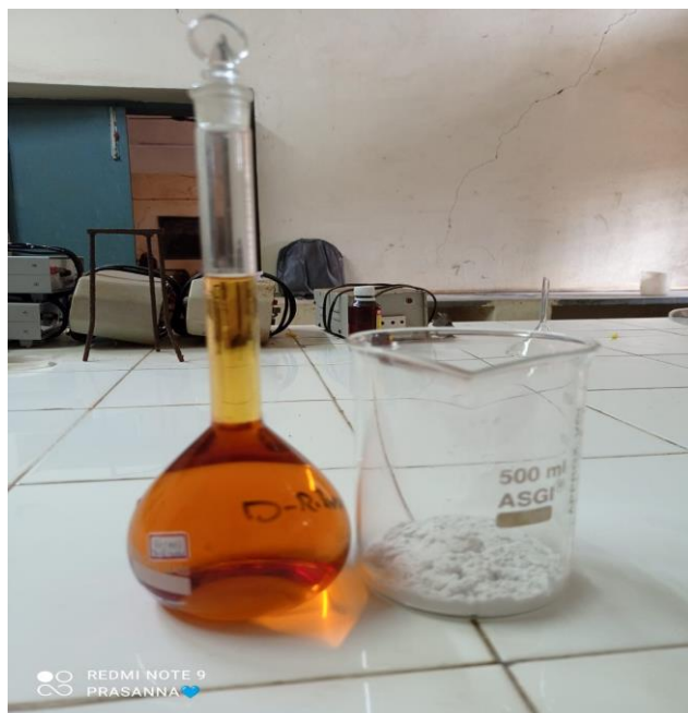
5 grams of Cellulose added to 100ml of Metal Ligand solution
