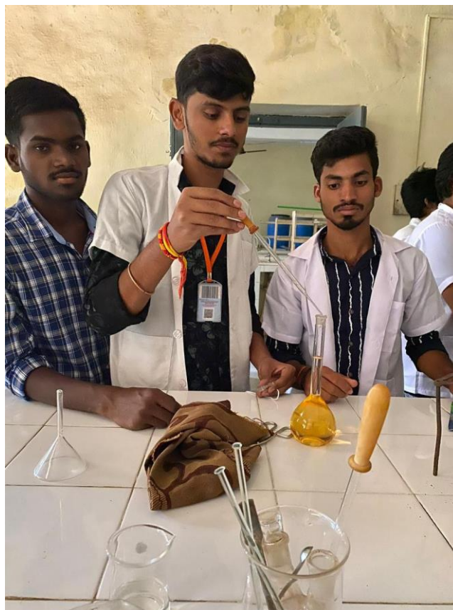
Preparing 250 ml of metal ligand solution using volumetric flask
