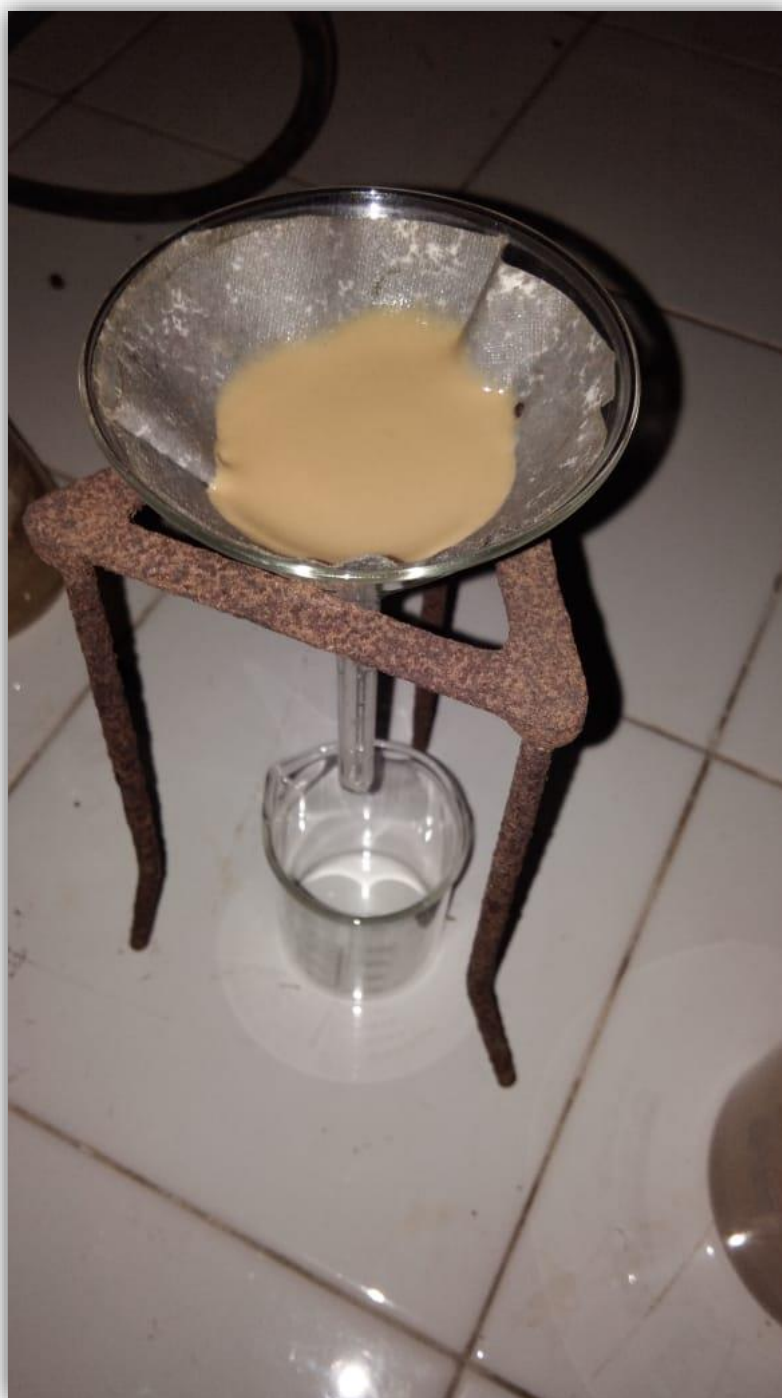
Filtering The Mixture using Whatman grade 1 filter paper and Again, three times by using Ultra-Pure water
