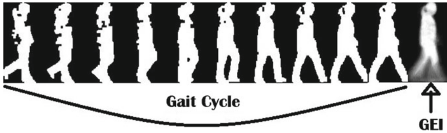
Fig. 4 GEI is mean of gait silhouettes over one gait cycle for CASIA A dataset
