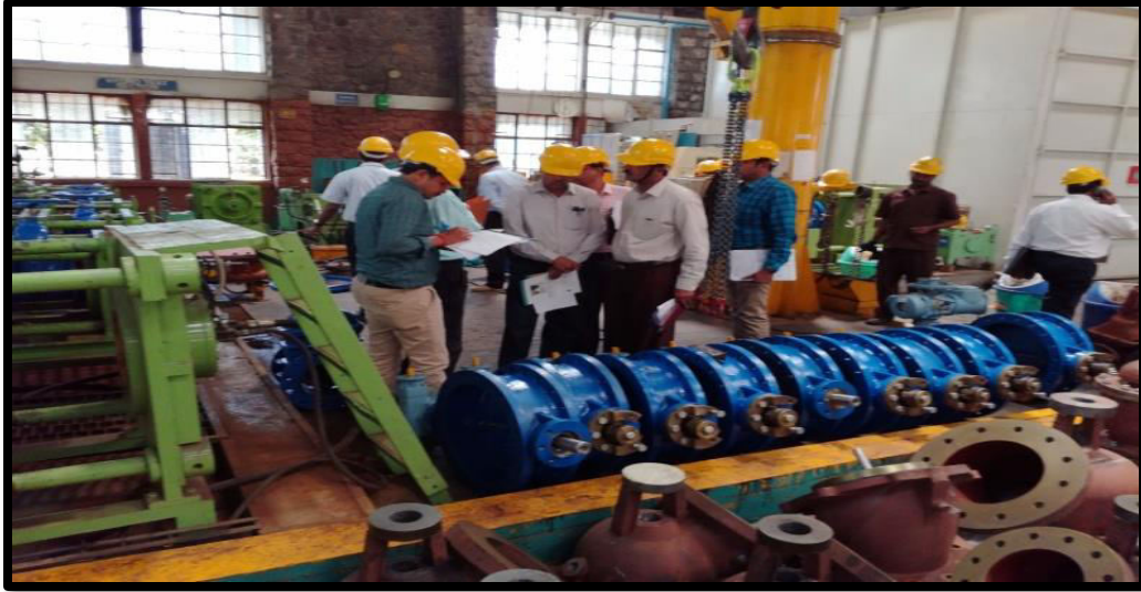
Inspection of valves at M/s KBL factory, Pune
