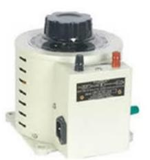
These types of transformers use a common winding for both primary and secondary windings. The autotransformer winding has three taps where the electrical connections are made. Autotransformers have the advantage of being smaller, lighter, and cheaper than typical transformers.
