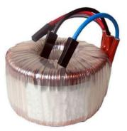
The toroidal core transformer uses a magnetic core which almost looks like a ring or donut called a toroidal. They are passive electronic components, consisting of a circular ring-shaped magnetic core of ferromagnetic material around which the wire is wound.
