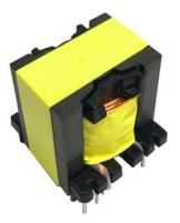
This type of transformer uses a magnetic core made of ferrite on which the windings of power transformers and other parts are made. Ferrite cores have high magnetic permeability, so they are used in high-frequency applications such as switch-mode power supplies.
