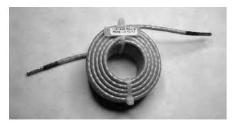
In this transformer, both the primary and secondary windings are set on a non-magnetic stripe. It has flux linkage in both the windings through the air. The mutual inductance in the air-core is low, which means the reluctance to be given to the generated flux is high in the air medium.
