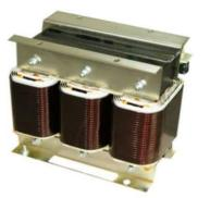
This type of transformer is used to transfer electrical power from an alternating current while isolating the powered device for safety reasons. The isolation transformer can provide galvanic isolation which means that no conductive path exists between the source and the load.
