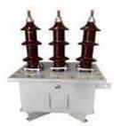
Potential transformers or voltage transformers are commonly used to reduce voltage levels. They cannot be used to supply natural power to a load and are used with voltmeters, watt-meters, frequency meters, circuit breakers tripping circuits, etc. In this, the primary winding is connected to the high voltage circuit and the secondary winding is connected to equipment or other circuits.
