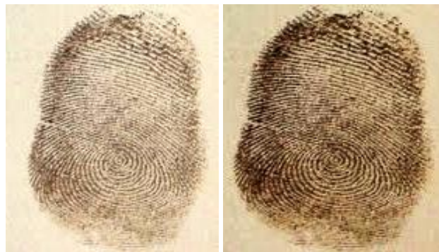
Figure 2: Development Using Iodine fuming-ethyl acetate method on A4 size paper.
