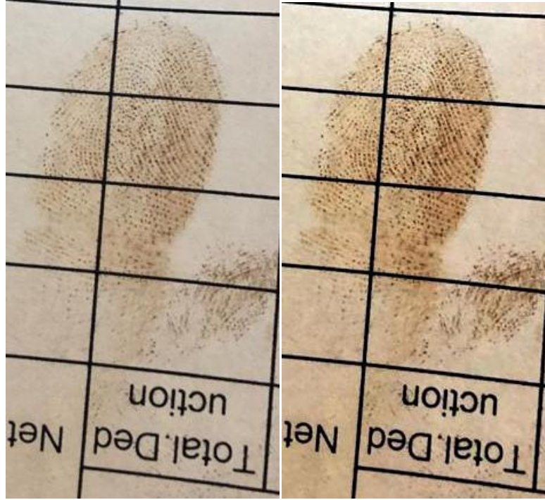
Figure 3: Development Using Iodine fuming-ethyl acetate method on scripted paper.
