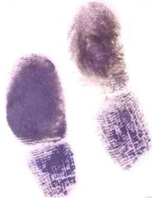
Figure 6: Development of latent finger print on paper
