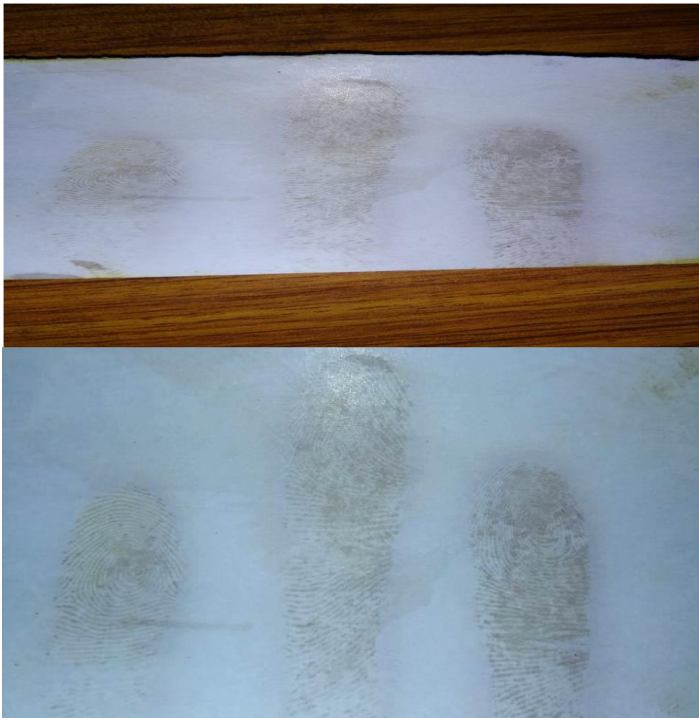
Figure 7: Development of latent finger print on Chart paper.
