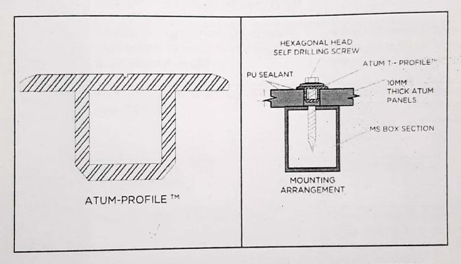
Sealant Specifications: 3M PU 540
